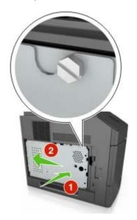
**6** Tighten the screws on the shield.
