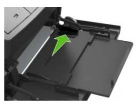
**Note:** Use the paper size indicators on the bottom of tray to help position the guides.
