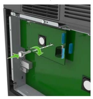
Note: Turn the screw clockwise, enough to hold the ISP in place, but do not tighten it yet.
