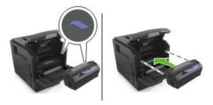
**Warning—Potential Damage:** When replacing a toner cartridge, do not leave the imaging unit exposed to direct light for an extended period of time. Extended exposure to light may cause print quality problems.
