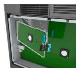
**Note:** Hold the ISP at an angle over the plastic bracket so that any overhanging connectors will pass through the ISP opening in the controller board cage.
