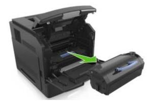
**3** Lift the blue handle, and then pull out the imaging unit from the printer.
