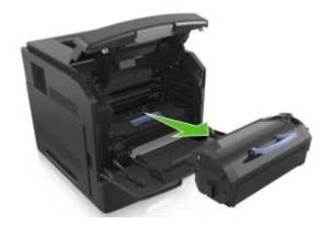
**3** Unpack the new toner cartridge, then remove the packing material, and then shake the cartridge to redistribute the toner.
