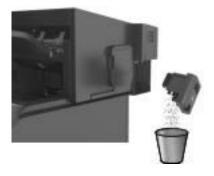
**3** Insert the emptied hole punch box back into the finisher until it *clicks* into place.
