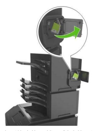
**2** Pull down the latch of the staple cartridge holder, and then pull the holder out of the finisher.
